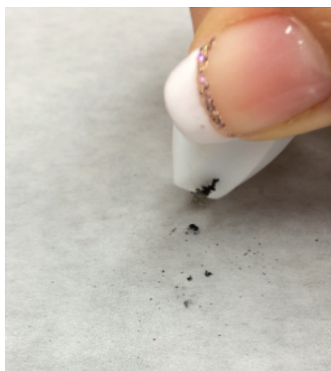
Figure A4.3. Pyrolyzed block copolymer gets attracted to permanent magnets.
